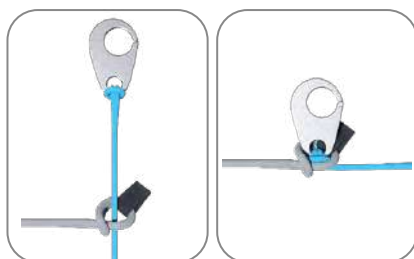
Diagram 1. Speed-bar connection by means of the Brummel hook.
