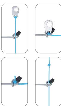
1. A knot is tied in the speed-bar cord and passed through the connector of the riser cord.
