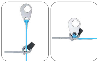
Diagram 1. Speed-bar connection by means of the Brummel hook. The blue line is from the harness, and the gray from the riser.
